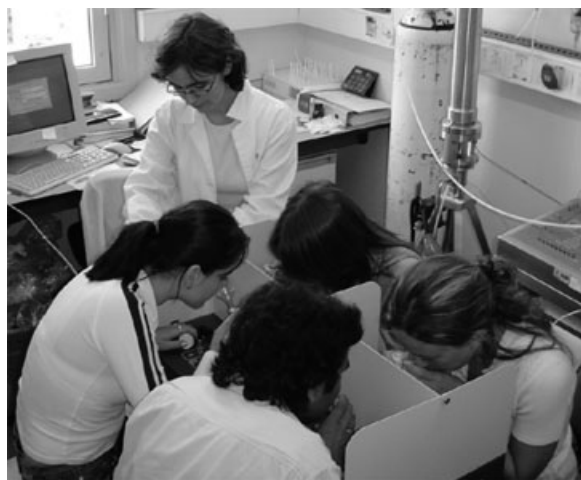
Figure 3. Measurement of odor threshold value using a panel of four people and an olfactometer.
